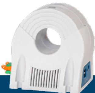
The frequency-selective DCTR B-X Hz PoE detects and evaluates residual currents at frequencies of 0 to 100 kHz with full reliability and displays them via the PoE interface in the DCTR Manager software. Constant monitoring of residual currents by the DCTR B-X Hz PoE provides information about the system's isolation and/or leakage current status. As per DIN VDE 0105-100/A1, this can be used to avoid repeat insulation tests, which can often be expensive.
